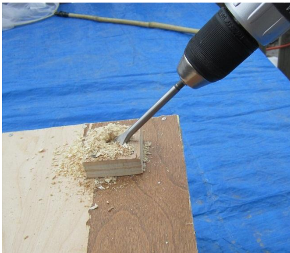
Photo #9: Drill entrance hole up at 45 degrees.
