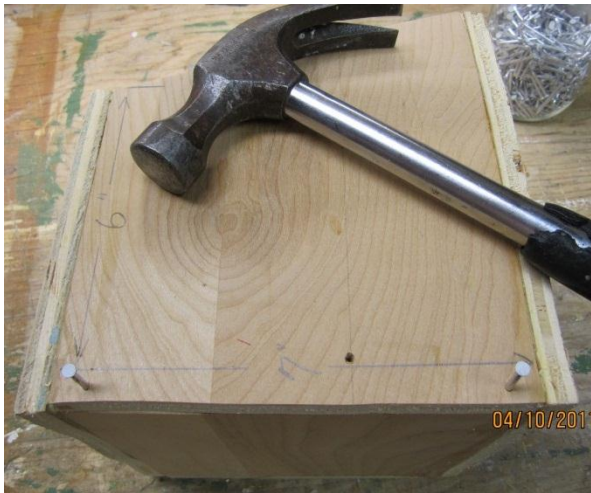
Photo #7: Ready to nail base to house.
