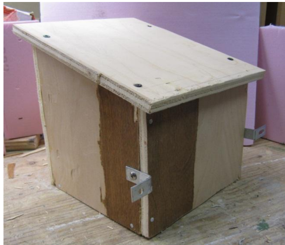
Photo #16: Shot showing mounting brackets at back of house.
